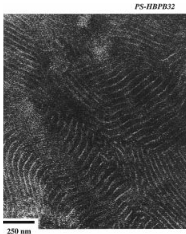
Figure 5. Representative lamellar morphology observed in TEM for LC block copolymer series. The sample shown is PS-HBPB32. Dark regions are polystyrene stained with \text{RuO}_4 and lighter regions are the LC copolymer.
